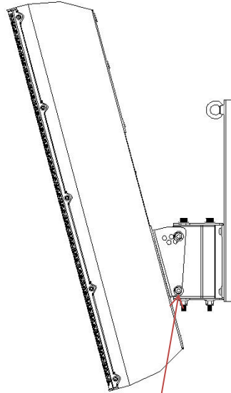
Figure 5 showing the tilt pivot bolt. This must be inserted first.
